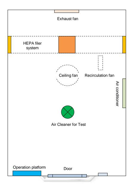
Figure 1 Schematic layout of the test chamber
